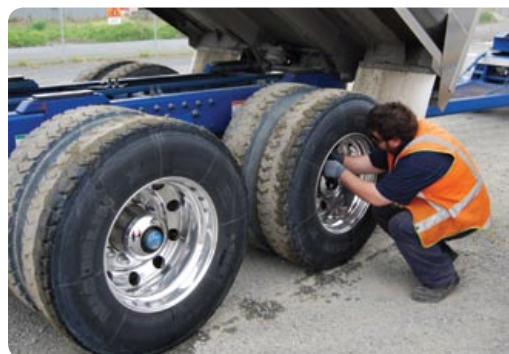
Operating tyres at optimal pressure can result in fuel savings of up to 3%.
