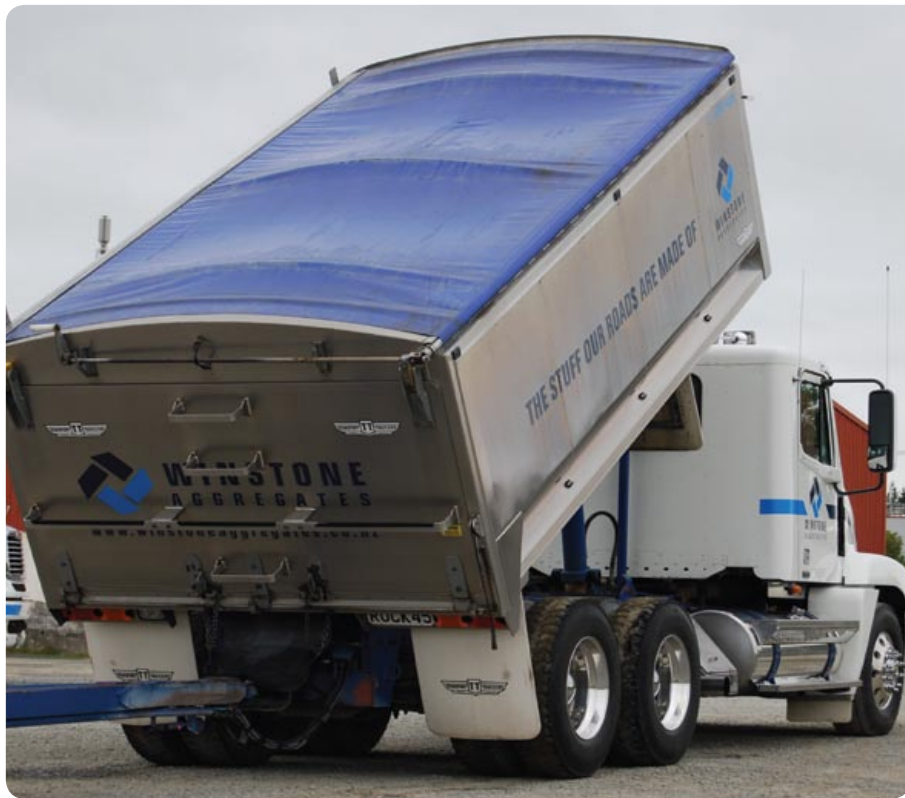
Covering trucks at all times can create energy savings of around 8%.
